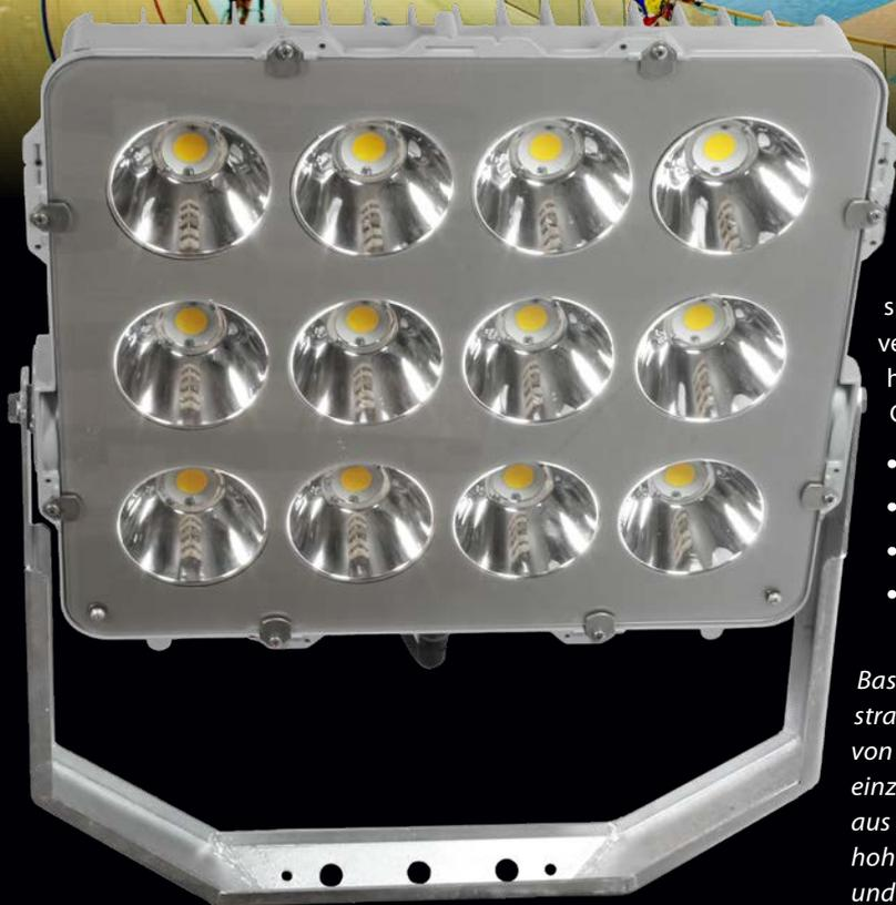
Based on the principle of reflection, the **PLUS OPTIC** with symmetrical beam offers the highest luminous efficiency for the lighting of amateur sports facilities and minor professional sports. Each individual LED is wrapped in its single reflector, in very high purity aluminum (99.99%) or vacuum metallized with high durability and efficiency, for better glare control (UGR and GR) and light distribution.
